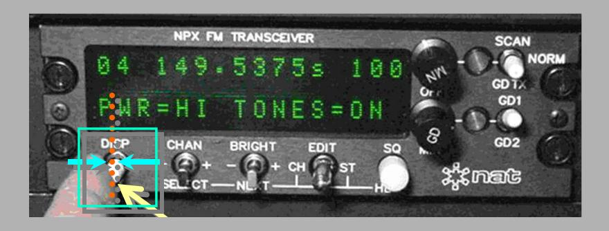
• Switch to the center is the Receive Display. This is the actual receive frequency for this "channel"
