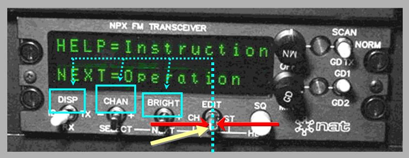
The position of the EDIT switch governs the way in which the other switches operate. This is a pull-type lockout toggle switch
