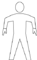
Arms extended with forearm perpendicular to ground. Palms facing body. HOT BRAKES
